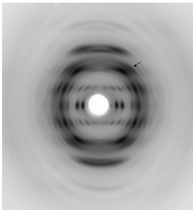
Figure 3. X-ray fiber diffraction pattern of the crystalline form of s-PPMS obtained by exposing an oriented sample of the mesomorphic form IV to cyclohexane vapors. The arrow indicates the presence of some residual mesomorphic form. Fiber axis direction is vertical.
