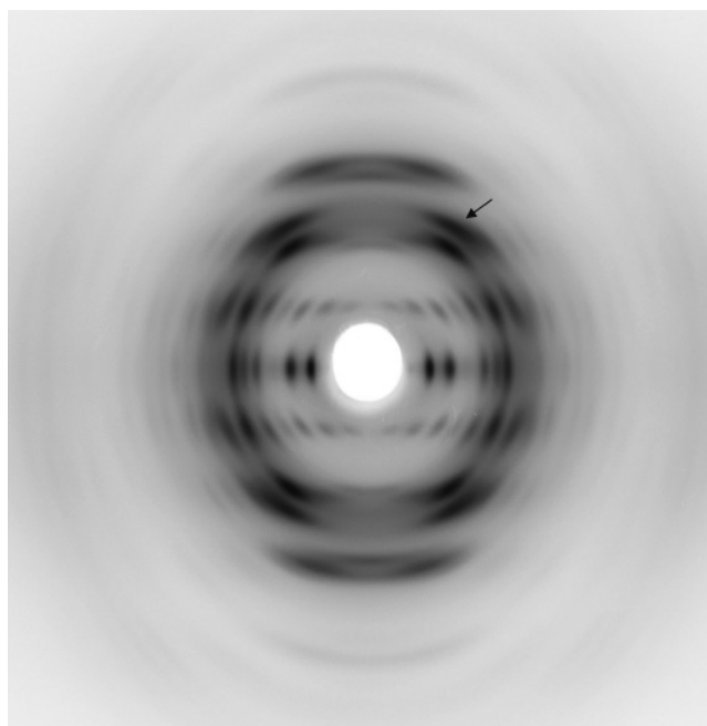
Figure 2. X-ray fiber diffraction pattern of the crystalline form of s-PPMS obtained by exposing an oriented sample of mesomorphic form IV to cyclohexanone vapors. The arrow indicates the presence of some residual mesomorphic form. Fiber axis direction is vertical.
